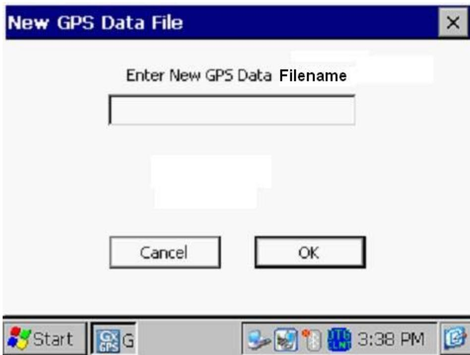
In the “Enter New GPS Data Filename” field, you can enter a name for the file in which the GPS position data will be stored.
